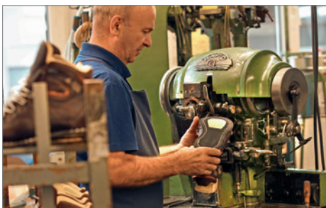
Setting a double seam
