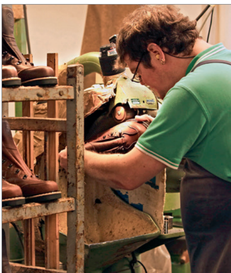
Milling the side of the sole
