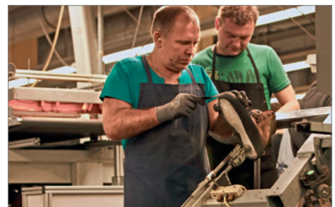
Applying the rubber rand
